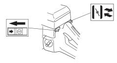
Use the same procedure as for starting a cold engine but without setting the choke control in the choke position. The correct choke/start throttle setting is obtained by moving the choke control to the choke position and then pushing it in again.
